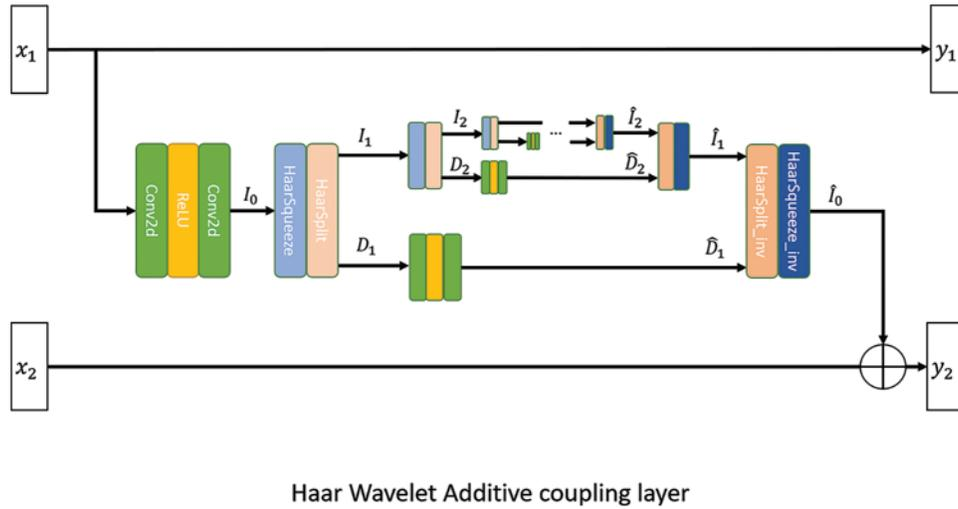
**Figure 2:** The structure of the proposed WAC layer. The left side is the inputs  $x_1, x_2$ . Notice  $x_1$  is used to generate features through multi-scale Wavelet transformation, which restores image features by levels in turn and then added on  $x_2$  as output  $y_2$ , and output  $y_1$  equals  $x_1$
