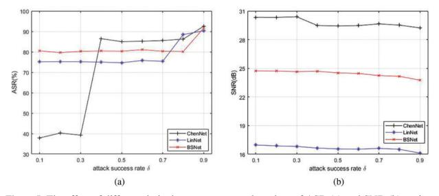
Figure 5: The effect of different desired success rates on the values of ASR (a) and SNR (b) against different detection networks
