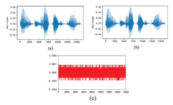
Figure 2: Clean cover before noise addition (a), diversified cover after noise addition (b), and the difference between them (c)
