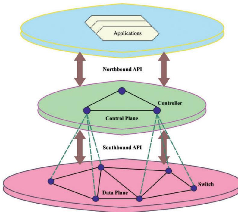
**Figure 1:** Process of SDN
