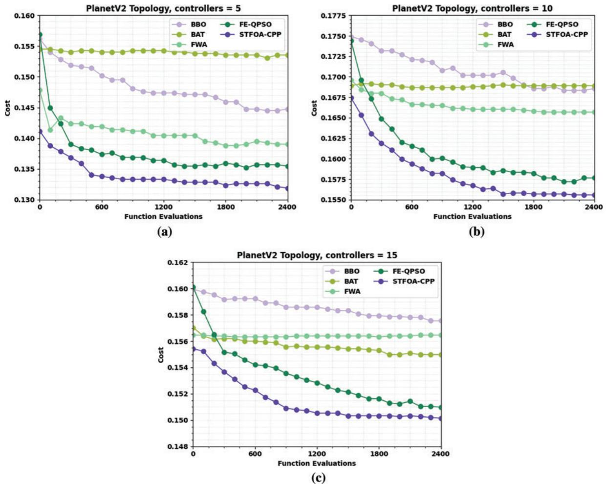
**Figure 2:** CP Cost analysis of STFOA-CPP approach based on PlanetV2 topology (a) controllers = 5, (b) controllers = 10, and (c) controllers = 15
