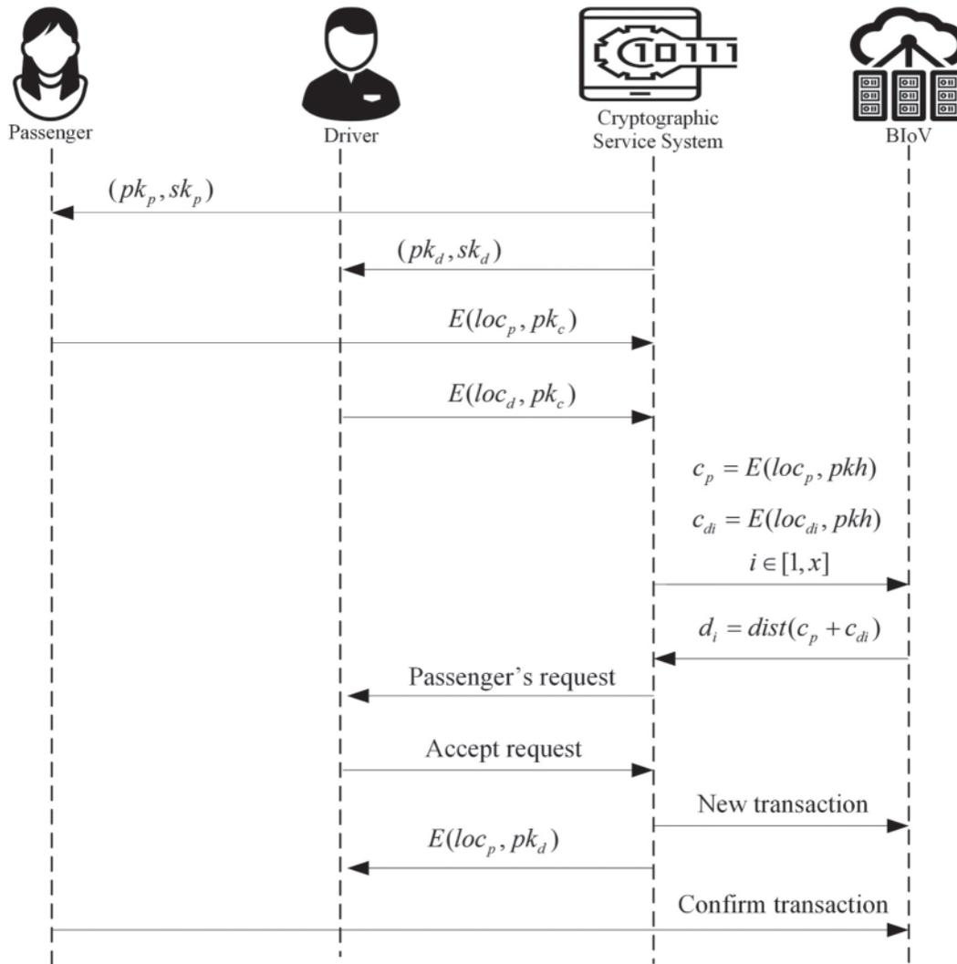
Figure 3: The processes of anonymity authentication for BIoV
