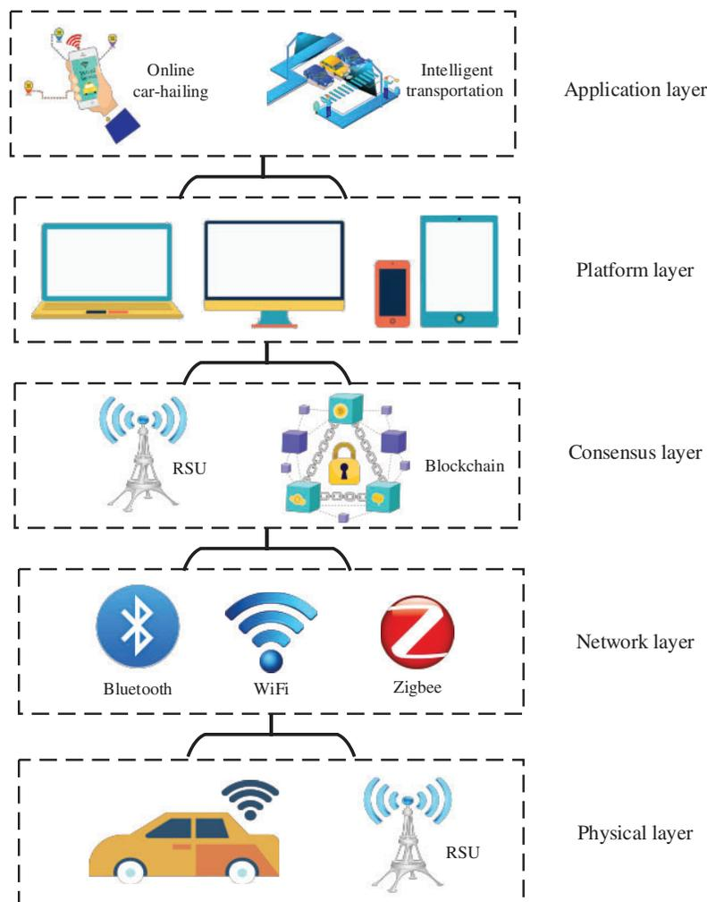
**Figure 2:** The architecture of BIoV
