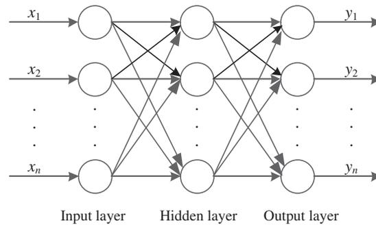
**Figure 3:** Topology of a BP network
