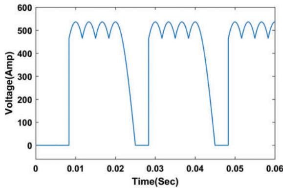
(a) Output voltage of VT1 with an open circuit
