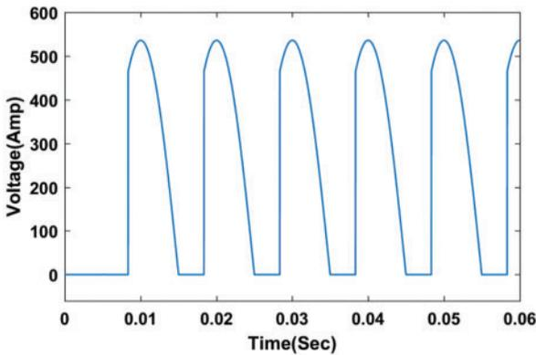
(c) Output voltage of VT1 and VT4 with an open circuit
