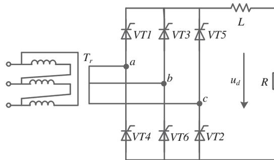
**Figure 1:** Three-phase bridge rectifier circuit
