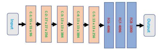
Figure 1: The general block diagram of the AlexNet structure
