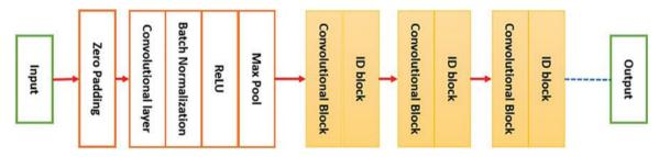
Figure 2: The block diagram of ResNet50
