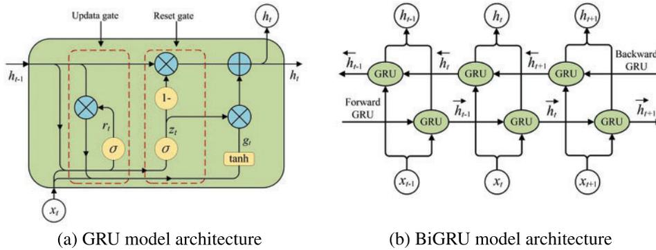
Figure 3: GRU model architecture
