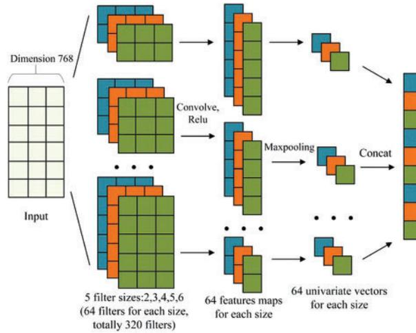
**Figure 4:** TextCNN model architecture
