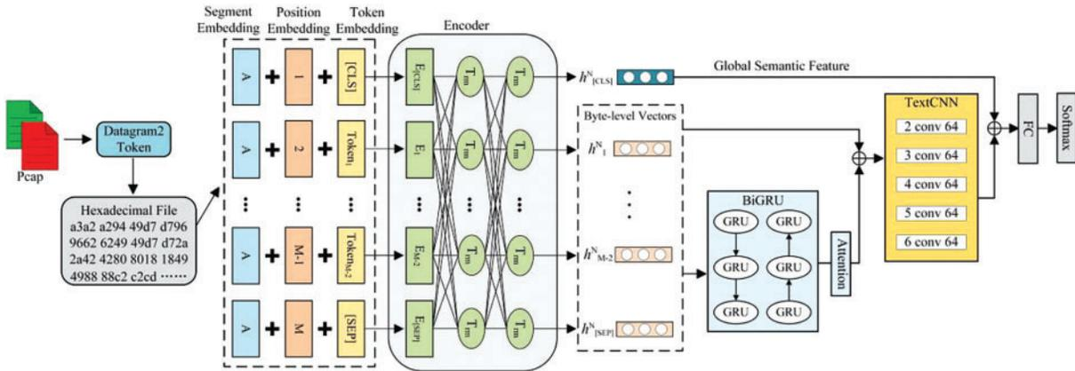
Figure 1: BSTFNet model architecture
