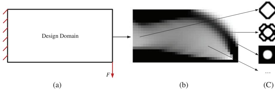
**Figure 1:** Multiscale topology optimization with non-uniform microstructures. (a) Structural design domain (b) Macrostructure (c) Microstructures
