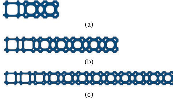
**Figure 5:** Multiple transition unit cells (a) 1 transition unit cell (b) 5 transition unit cells (c) 10 transition unit cells
