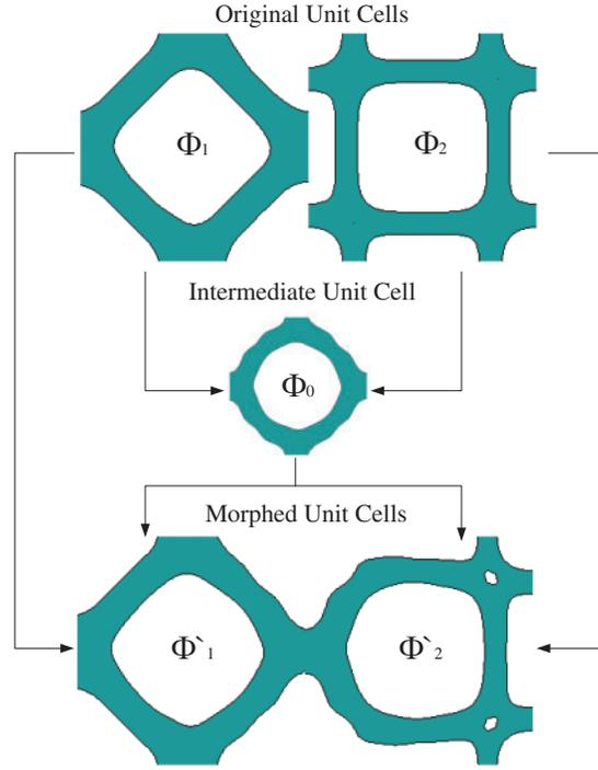
**Figure 6:** Morphed unit cells with intermediate unit cell
