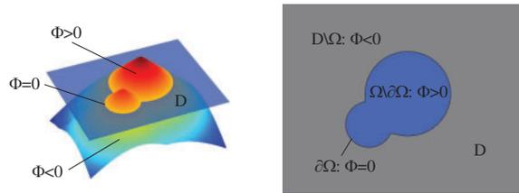
**Figure 2:** Structural boundary and the corresponding LSF
