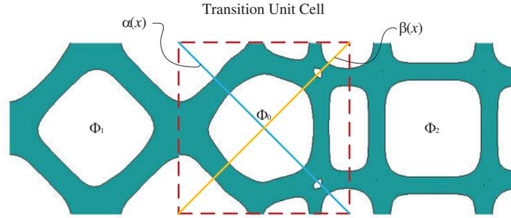
**Figure 4:** Interpolated transition unit cells with LSF  $\Phi_0$
