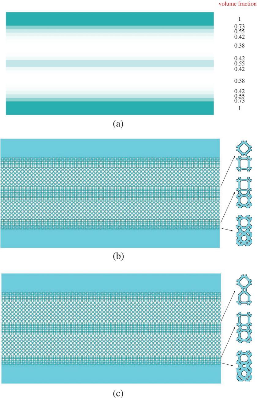
**Figure 13:** Two-scale topology optimization of layered beam (a) macro-scale topology optimization (b) micro-scale topology optimization without interpolation algorithm (c) micro-scale topology optimization with an interpolation algorithm
