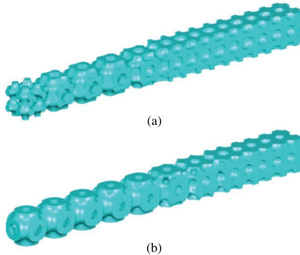
**Figure 10:** Optimized 3D FGM with volume fractions ranging from 0.35 to 0.8 (a) maximum bulk modulus (b) maximum shear modulus
