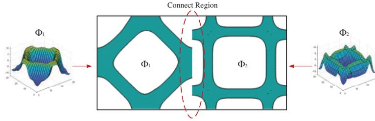
**Figure 3:** Unit cells with maximum values on shear modulus (left) and bulk modulus (right) in terms of volume fraction is 0.4
