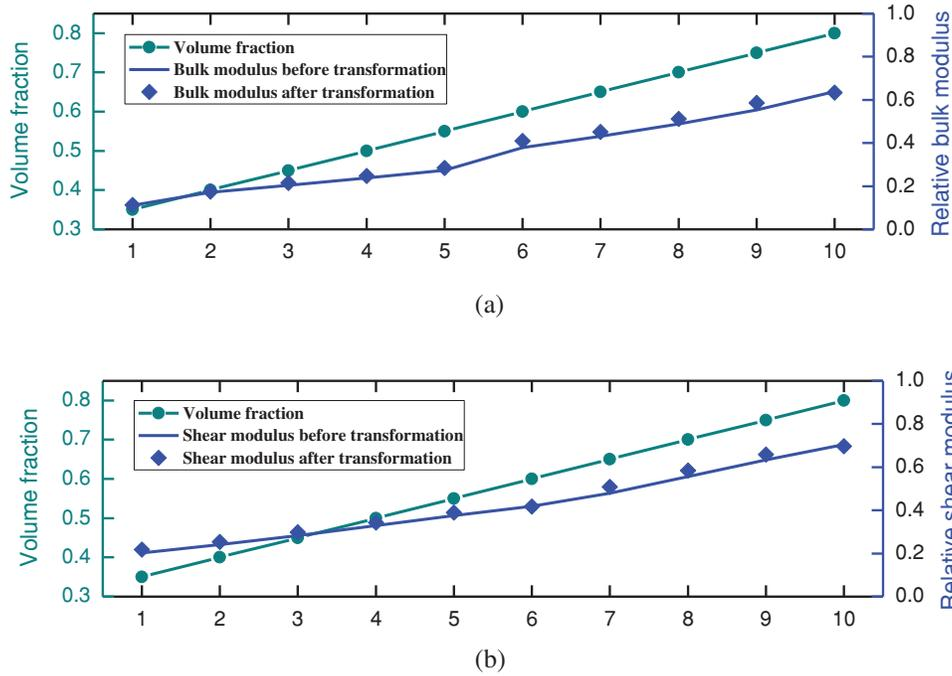
**Figure 11:** Comparison of properties before and after transformation (a) maximum bulk modulus (b) maximum shear modulus
