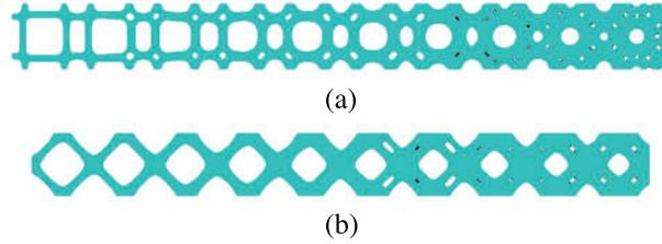
**Figure 8:** Optimized 2D FGM with volume fractions ranging from 0.35 to 0.8 (a) maximum bulk modulus (b) maximum shear modulus
