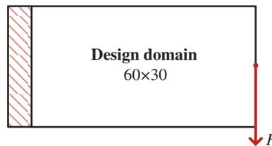
**Figure 12:** Design domain of the layered cantilever beam
