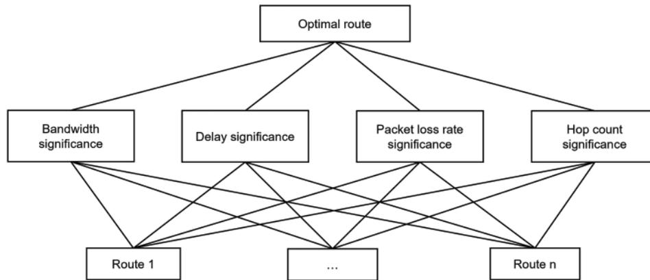
**Figure 3:** A hierarchical model for path optimization
