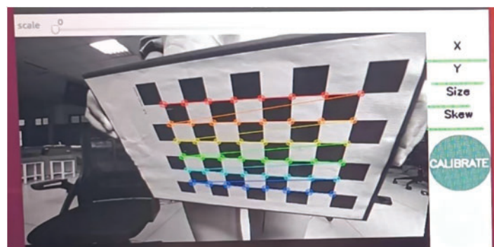
Figure 10: Camera intrinsic parameter calibration process
