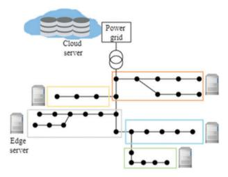
Figure 3: IEEE 33 bus model based on simulation scenario
