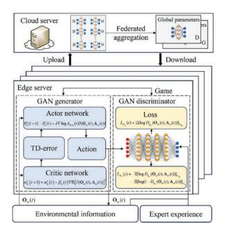
Figure 2: Framework of cloud-edge collaborative FGAN with long-term constraint violation sensitiveness
