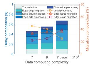
Figure 10: Delay composition and migration composition vs. data computation complexity
