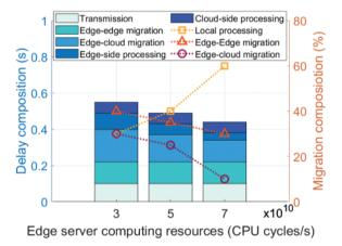
Figure 9: Delay composition and migration composition vs. edge server computing resources
