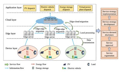
Figure 1: Multi-flow integrated energy aggregation dispatch framework based on cloud-edge collaboration
