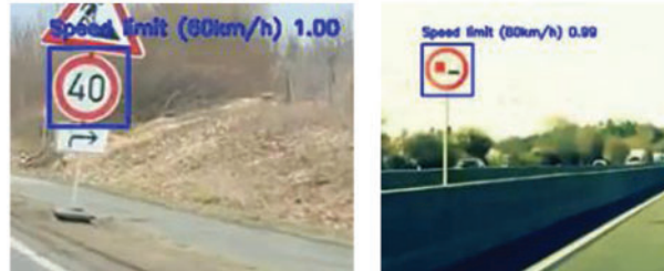
Figure 4: Examples of signs incorrectly recognized by the SLR system
