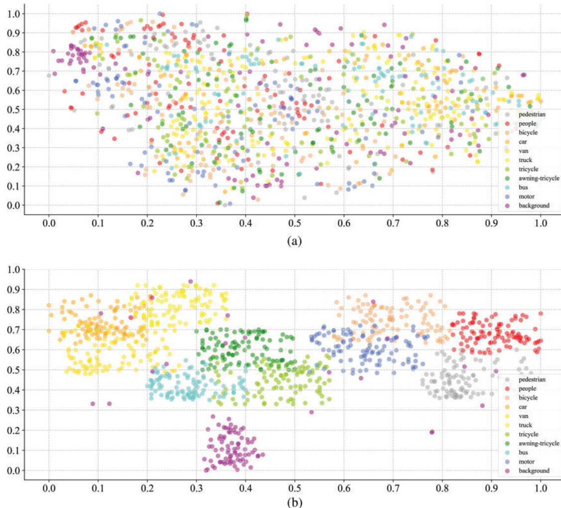
Figure 4: Visualization results of the encoded feature distribution from ResNet50. (a) Without momentum contrast learning. (b) With momentum contrast learning
