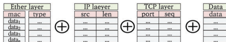
Figure 4: Network packet layer encoding (len, length; seq, sequence; src, source)
