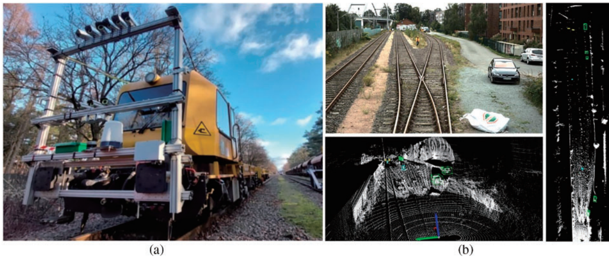
Figure 5: OSDaR23 acquisition equipment and part of the data. (a) Dataset acquisition equipment, (b) Example of dataset
