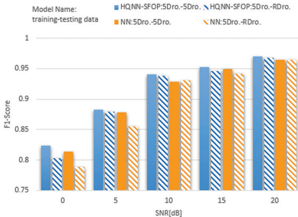
Figure 7: F1-score of HQNN-SFOP, NN for five drones datasets and random drones datasets at different SNRs
