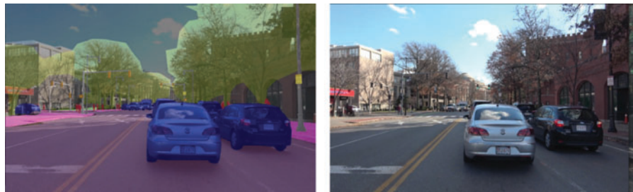
Figure 1: Example of semantic segmentation for autonomous driving: The left image depicts the original scene, while the right image shows the result of semantic segmentation
