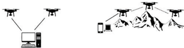
Figure 8: FANET devices managed by a non-mobile device vs. managed by mobile device
