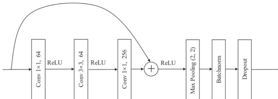
Figure 4: Basic CNN block
