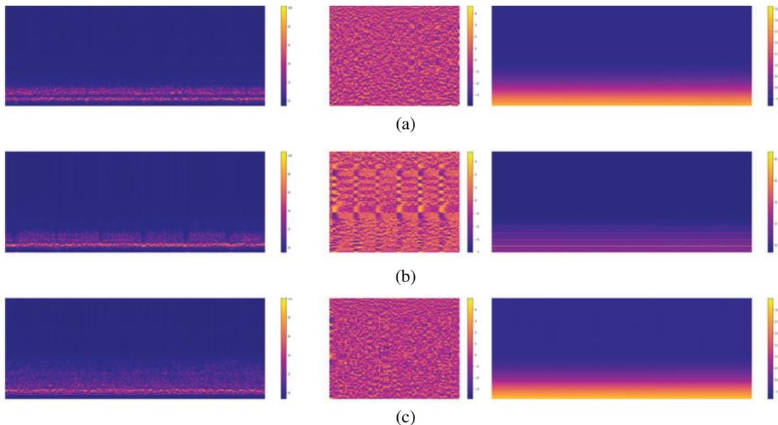
**Figure 3:** STFT spectra and MFCC of normal, cracking, and rubbing AE signals. (a) Normal. (b) Cracking. (c) Rubbing
