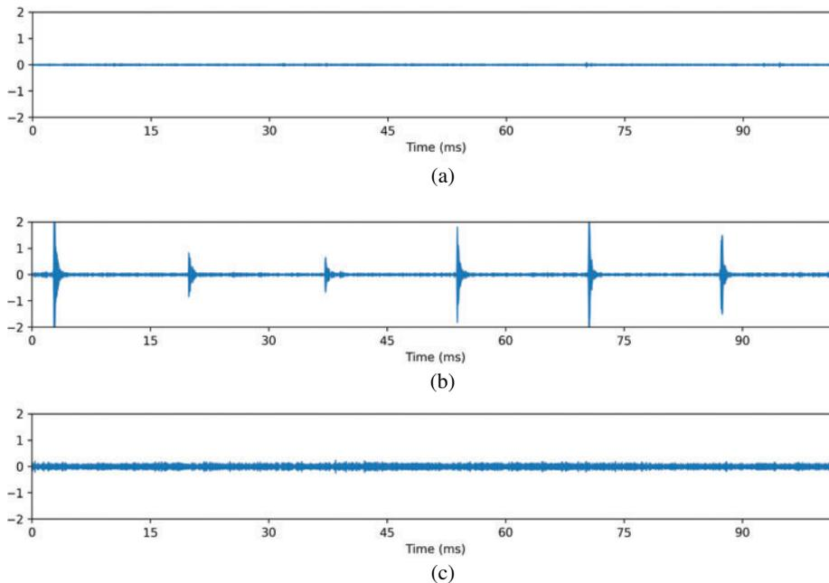
**Figure 6:** The database samples. (a) Normal. (b) Cracking. (c) Rubbing
