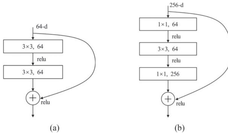
**Figure 1:** The ResNet Block structure. (a) a ResNet-34 building block. (b) a ResNet-50/101/152 bottleneck building block
