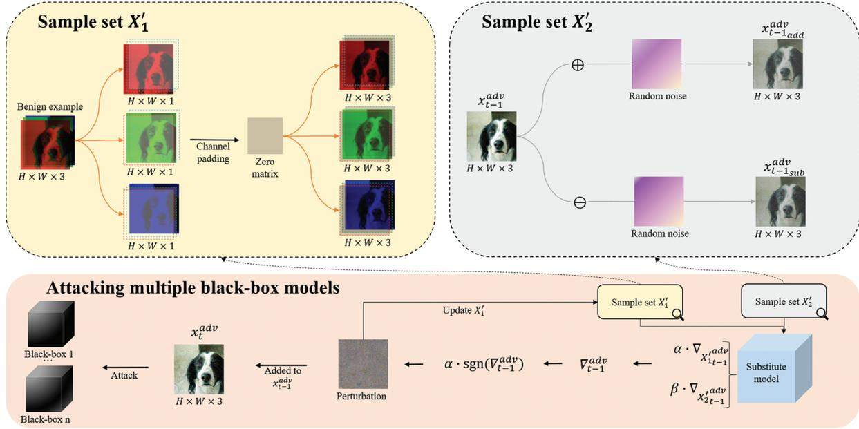
**Figure 2:** The framework of CDAM, where  $H$  denotes the image height and  $W$  denotes the image width,  $\text{sgn}$  is the sign function,  $x_{t-1}^{adv}$  is the adversarial example at  $t - 1$ -th iteration,  $\oplus$  denotes element-wise add,  $\ominus$  denotes element-wise minus. The adversarial examples generated by CDAM can attack multiple black-box models
