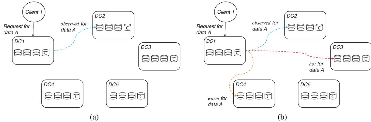
Figure 2: Data placement (a) without *hot*, *warm* (b) with *hot*, *warm*
