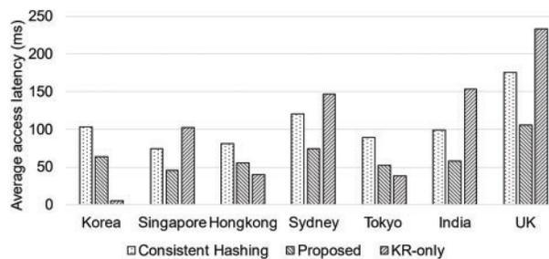
**Figure 3:** Average latency of client accessing the distributed storage
