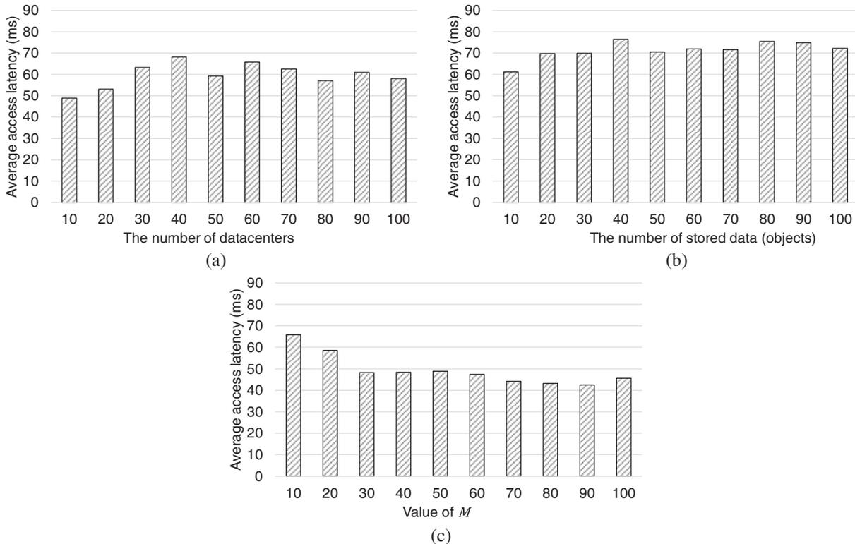
**Figure 4:** Average latency of client accessing the distributed storage with varying parameters
