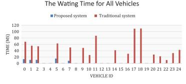
Figure 13: The waiting time for each vehicle in the fourth scenario
