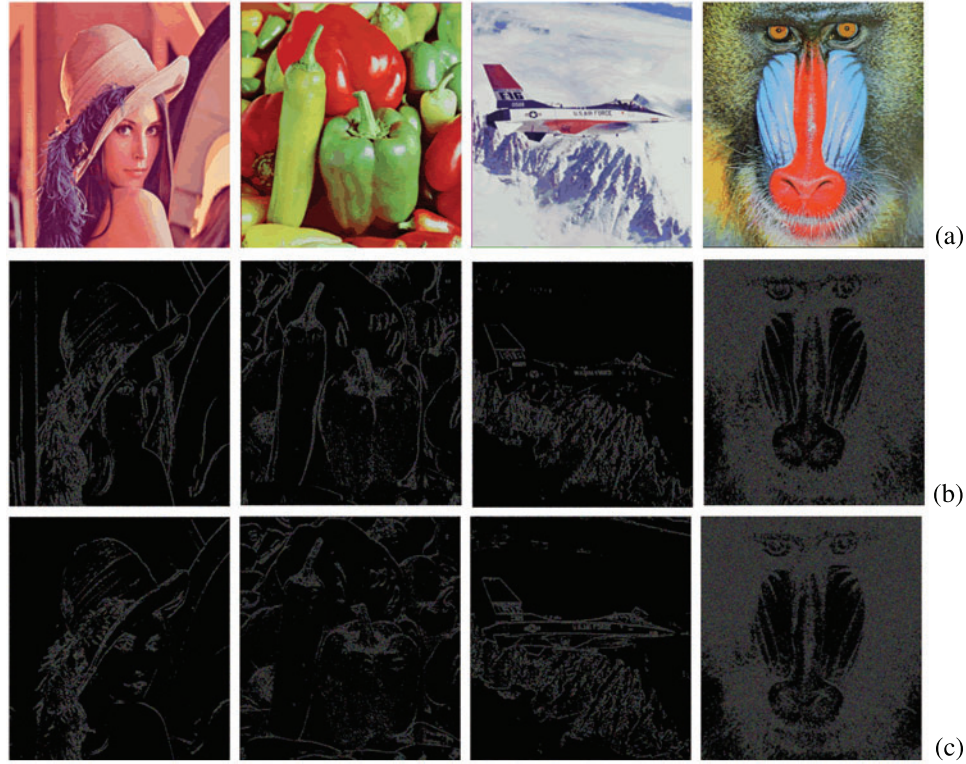
Figure 5: a) Original test images, b) Message-watermark images obtained using vertical edges, c) Message-watermark images obtained using horizontal edges
