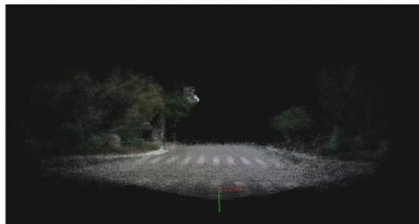
(D) Front view of cloud point map constructed by RO-SLAM
