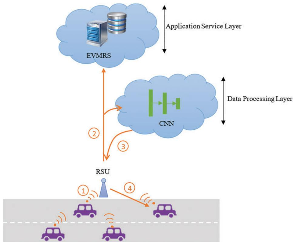
**Figure 1:** The proposed update model of the intrusion detection system
