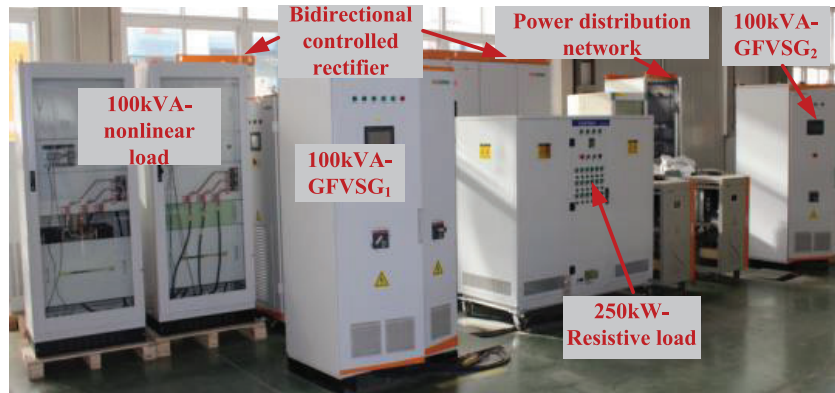
Figure 7: Energy storage microgrid system platform
