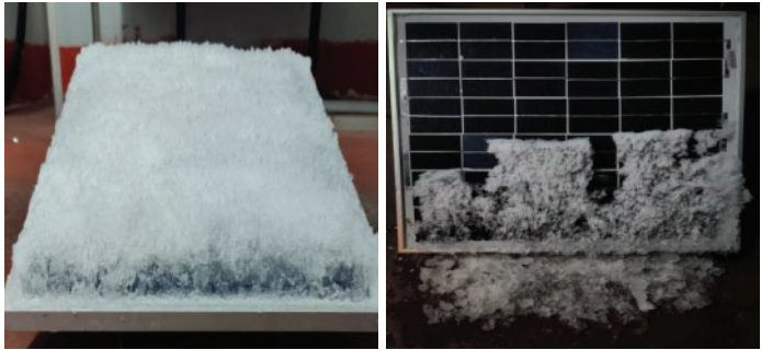
(d) snow accumulation and melting/shedding on PV modules obtained from the artificial climate laboratory.
