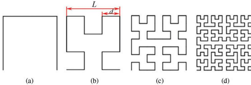
**Figure 2:** Hilbert fractal curves of different orders: (a) 1st-order curve; (b) 2nd-order curve; (c) 3rd-order curve; (d) 4th-order curve
