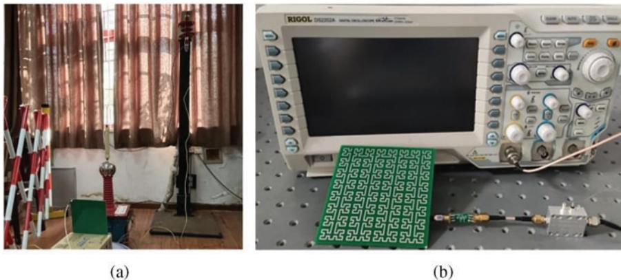
Figure 14: Images of the experimental platform: (a) PD signal generation component; (b) PD signal detection component
