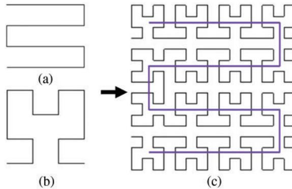
**Figure 4:** Design process for the proposed serpentine-Hilbert unit (SHU) antenna (a) 2nd-order; (b) 2-layer SHU curve; (c) wire component of length  $s$  connecting Hilbert fractal elements
