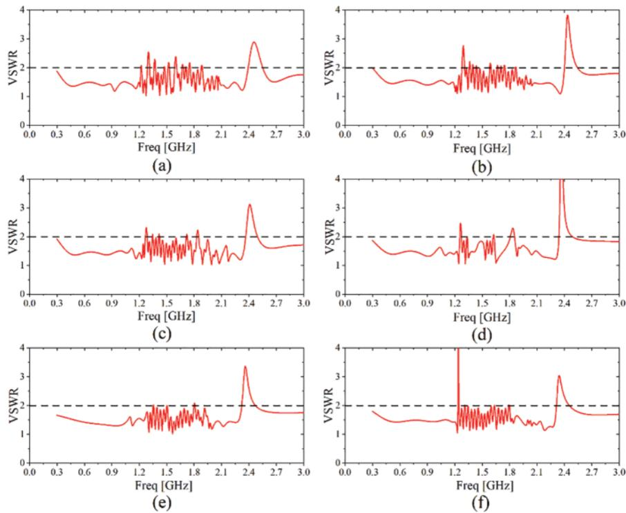
**Figure 9:** VSWR values of 2nd-order, 4-layer SHU antennas with different spacing values  $s$  as a function of frequency: (a)  $s = 1.8$  mm; (b)  $s = 2.1$  mm; (c)  $s = 2.4$  mm; (d)  $s = 2.7$  mm; (e)  $s = 3.0$  mm; (f)  $s = 3.3$  mm
