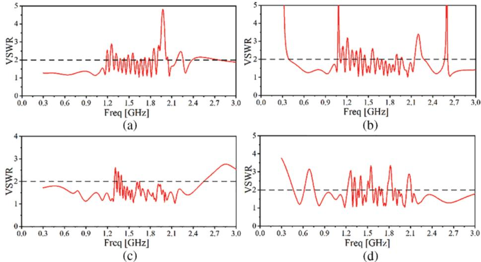
**Figure 6:** VSWR values of SHU antennas composed of 2nd-order Hilbert units with different numbers of serpentine layers as a function of frequency: (a) 2 serpentine layers; (b) 3 serpentine layers; (c) 4 serpentine layers; (d) 5 serpentine layers
