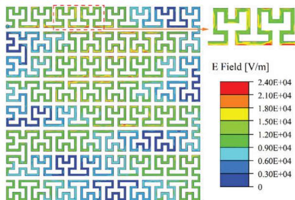
**Figure 7:** Electric field distribution obtained for a 2nd-order, 4-layer SHU antenna
