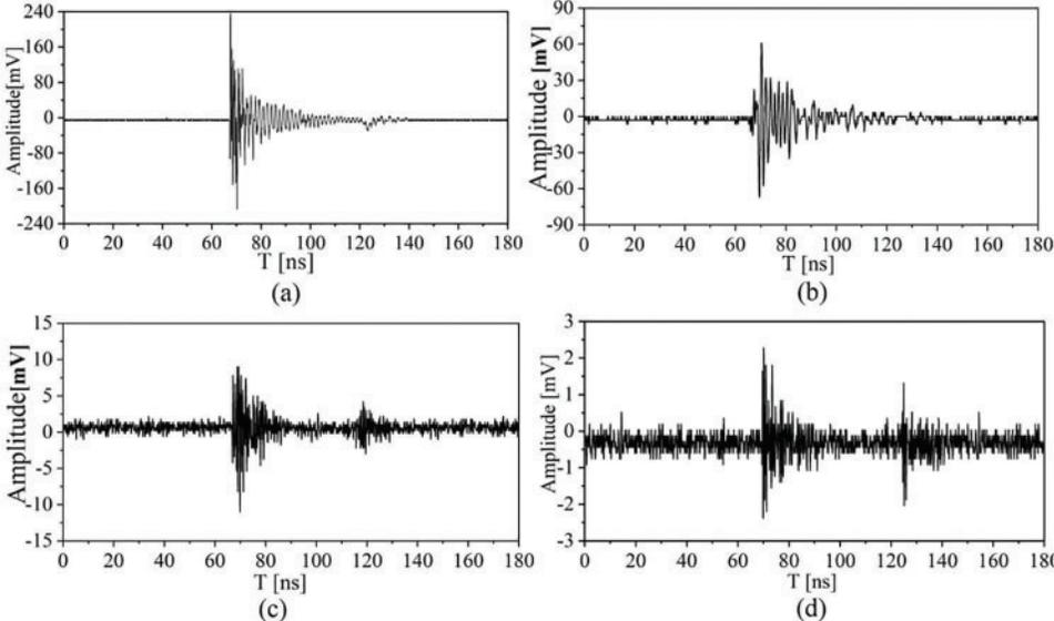
**Figure 16:** Time-domain waveforms of PD signals captured by the 2nd-order, 4-layer SHU antenna positioned at different detection distances  $D$  from the PD source: (a)  $D = 1$  m; (b)  $D = 2$  m; (c)  $D = 5$  m; (d)  $D = 8$  m
