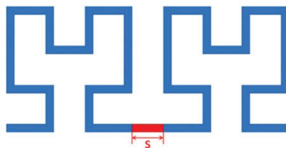
**Figure 8:** The spacing  $s$  of the Hilbert fractal elements
