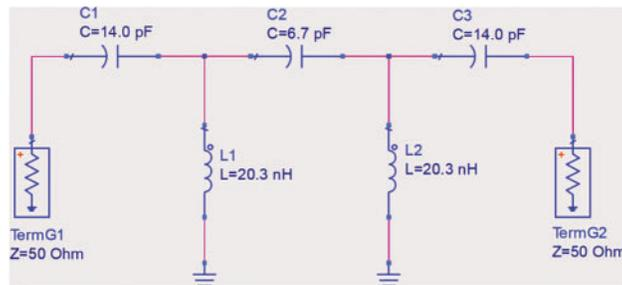
Figure 13: The structure and parameters of high-pass filter
