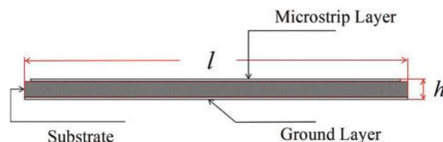
**Figure 1:** Schematic illustrating the microstrip patch antenna model
