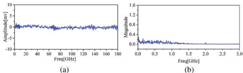
Figure 15: Experimental environmental noise: (a) The time-domain waveform; (b) The frequency-domain waveform
