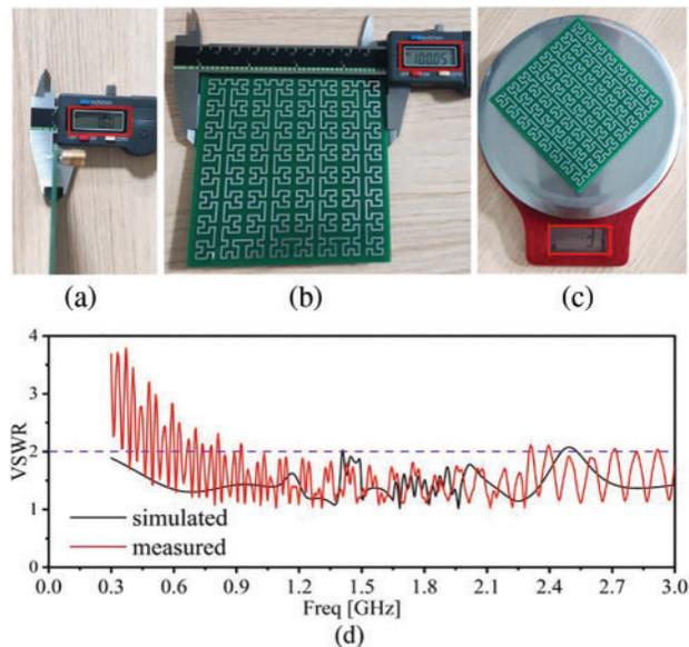
**Figure 11:** Prototype 2nd-order, 4-layer SHU antenna with  $s = 3.0$  mm fabricated according to the specifications listed in Table 1 using standard PCB technology: (a) side view; (b) front view; (c) weight; (d) VSWR curves obtained from simulation and experimental measurements
