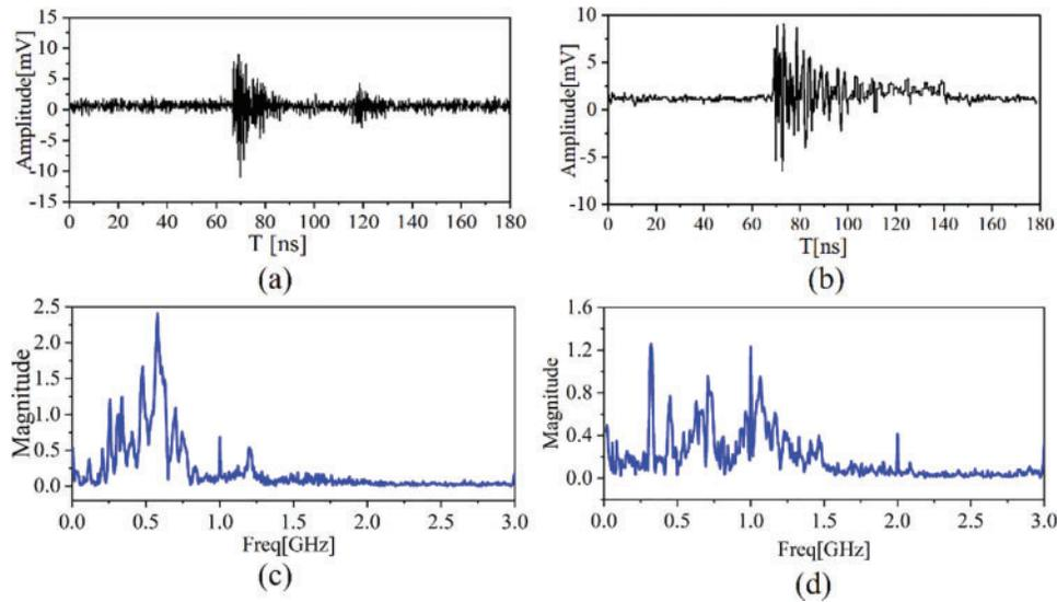
**Figure 17:** (a) The time-domain waveform diagram of 2nd-order, 4-layer SHU antenna; (b) The frequency-domain waveform diagram of 2nd-order, 4-layer SHU antenna; (c) The time-domain waveform diagram of the classical 4th-order Hilbert fractal antenna; (d) The frequency-domain waveform diagram of the classical 4th-order Hilbert fractal antenna
