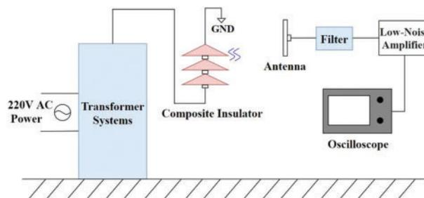
**Figure 12:** Schematic illustrating the experimental platform employed in the PD detection tests
