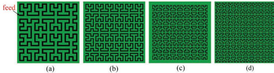
**Figure 5:** SHU antennas with 2nd-order Hilbert units and multiple-layer serpentine arrangements considered in the optimization process: (a) 2 serpentine layers; (b) 3 serpentine layers; (c) 4 serpentine layers; (d) 5 serpentine layers
