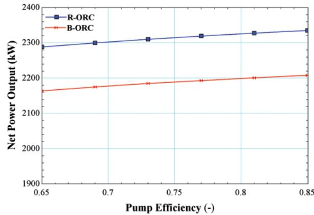
**Figure 9:** Impact of pump efficiency on net power
