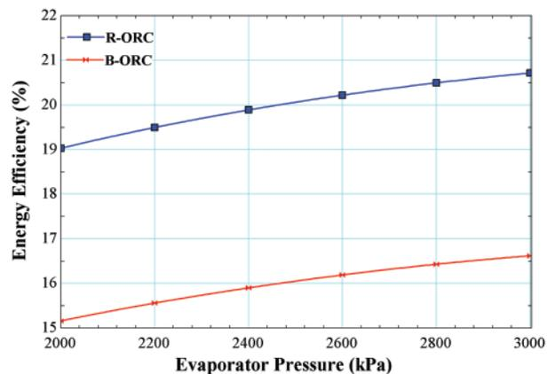
**Figure 4:** Effect of evaporator pressure on energy efficiency
