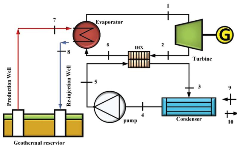
**Figure 2:** Schematic of regenerative ORC (R-ORC)
