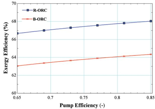
**Figure 11:** Effect of pump efficiency on exergy efficiency
