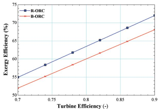
**Figure 8:** Impact of turbine efficiency on exergy efficiency
