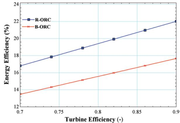
**Figure 7:** Impact of turbine efficiency on energy efficiency
