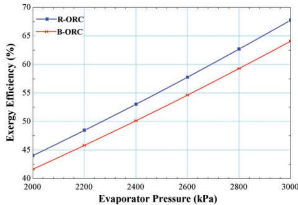
**Figure 5:** Effect of evaporator pressure on exergy efficiency
