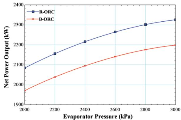
**Figure 3:** Impact of evaporator pressure on net power output
