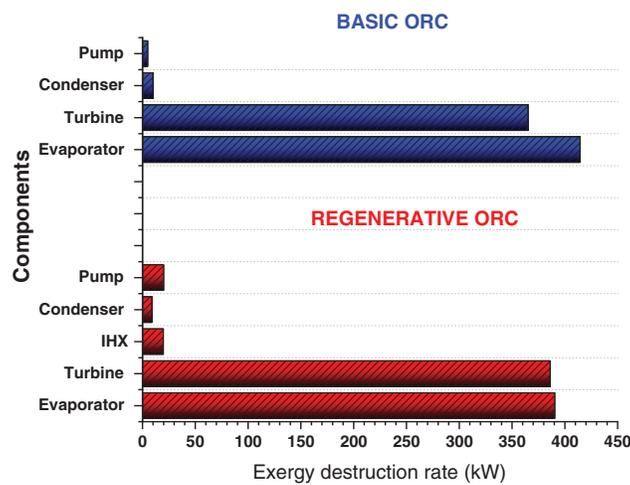
**Figure 12:** Exergy destruction rate in components of basic and regenerative ORC at optimal operating conditions
