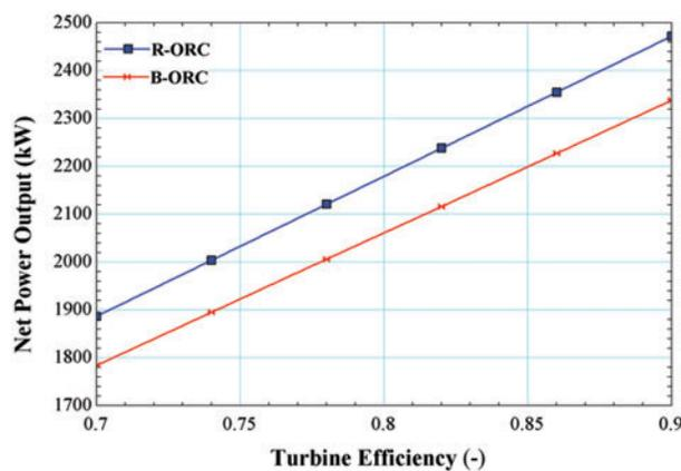
**Figure 6:** Impact of turbine efficiency on net power output
