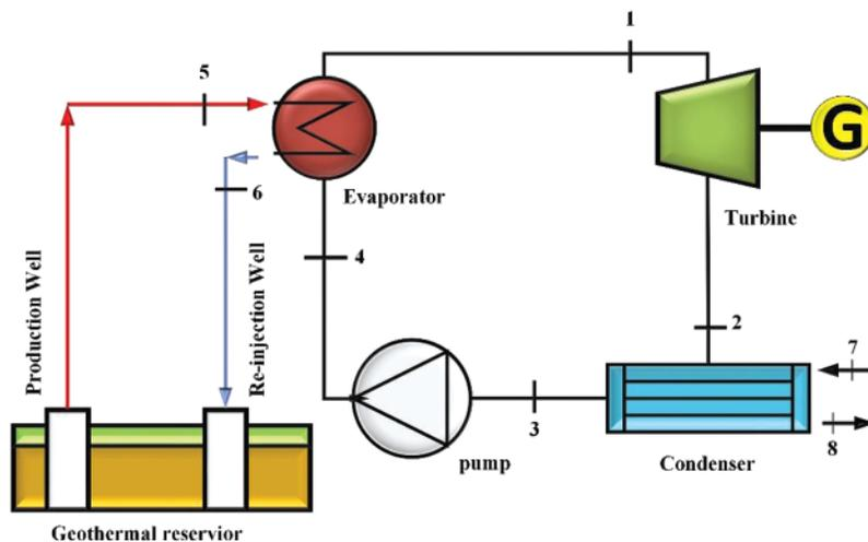
**Figure 1:** Schematic of basic ORC (B-ORC)
