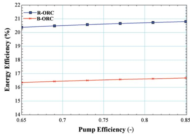
**Figure 10:** Impact of pump efficiency on energy efficiency
