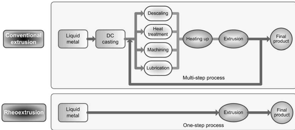
Figure 8: A comparison between rheoextrusion and conventional extrusion processes.
