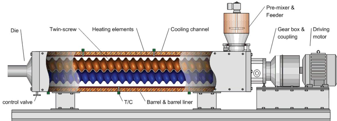
Figure 7: Schematic illustration of a prototype experimental rheoextruder
