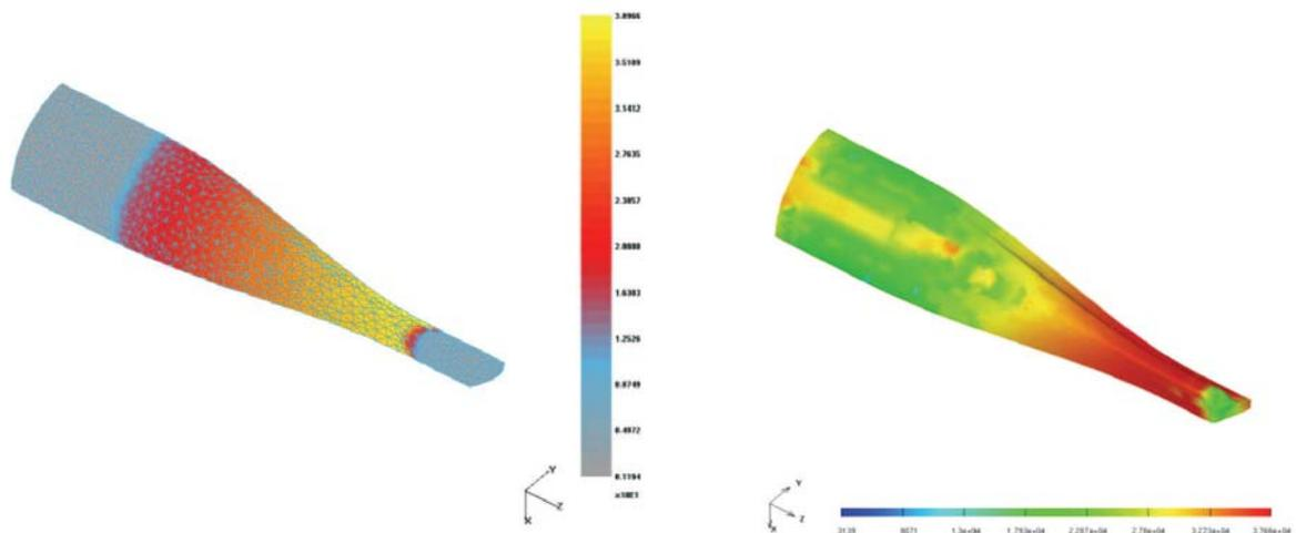
Figure 2: Effective stress distribution for a streamlined die extrusion simulation, left for DEFORM-3D<sup>®</sup>, right for MSC SuperForge (Mehta et al., 2000)
