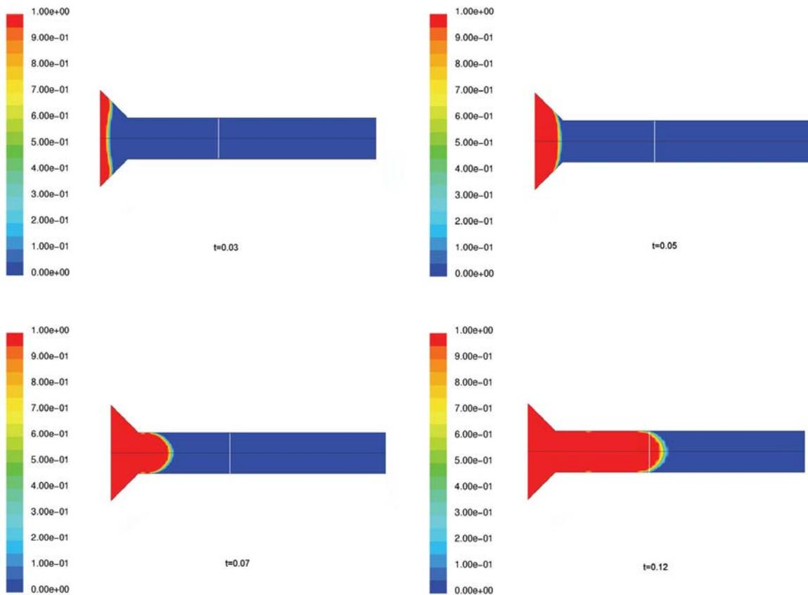
Figure 10: Simulation of filling process in die extrusion at different time steps.
