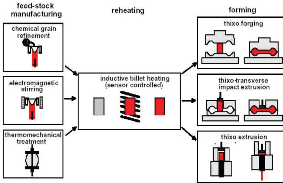
Figure 5: Process of thixo-route forming (Kopp et al., 1999).
