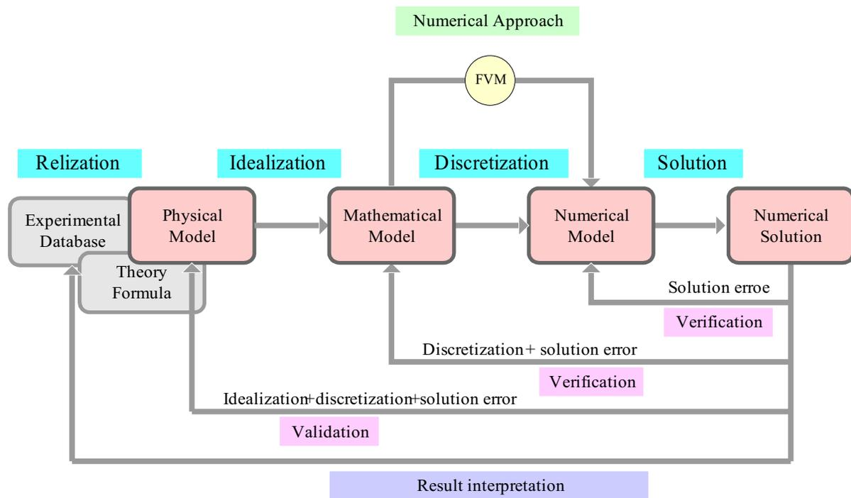
Figure 9: Schematic flowchart of simulation approach strategy
