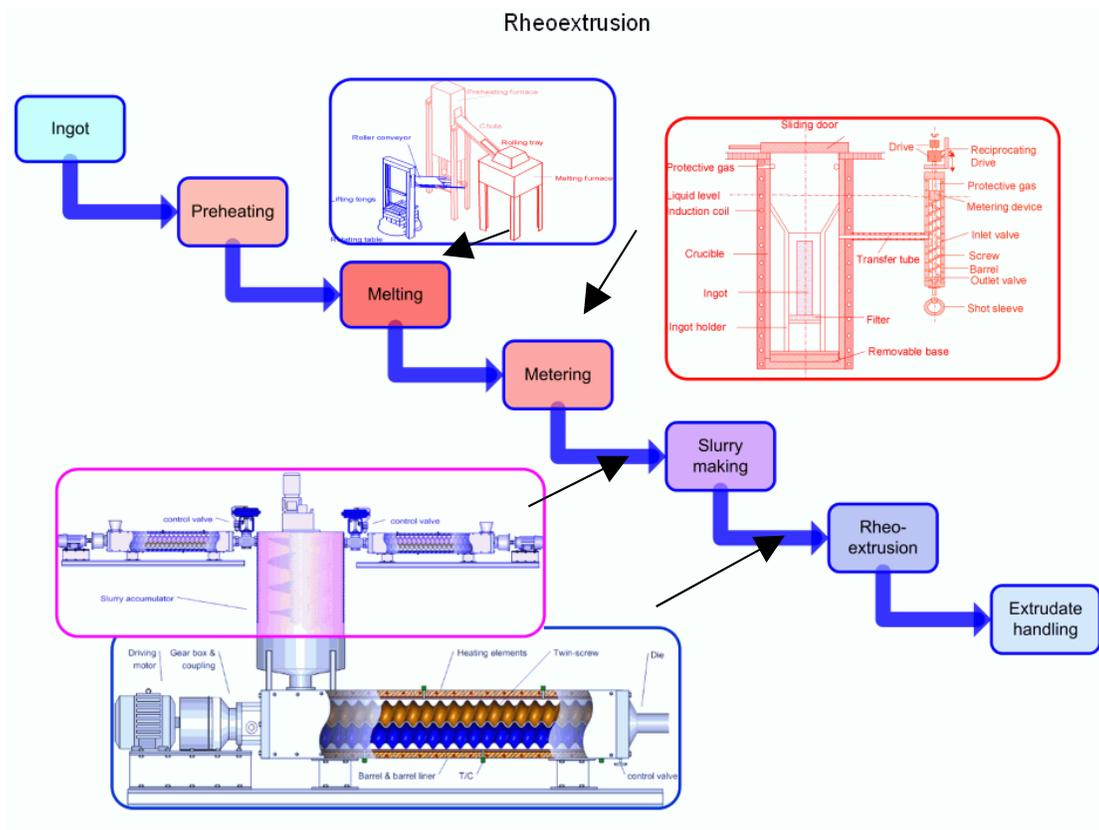
Figure 15: Flowchart of rheoextrusion process for industrial applications
