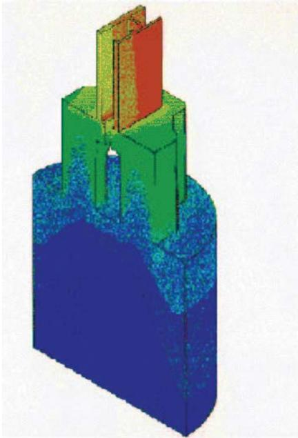
Figure 3: Fidap simulation of aluminium extrusion to improve porthole die design (Skauvik, 1999)
