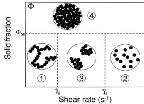
Figure 4-b: Structure of the suspension in the semi-solid phase-space. 1-gel, 2-suspension of individual particles, 3-suspension of clusters, 4-compact arrangement (Perez et al., 2000).
