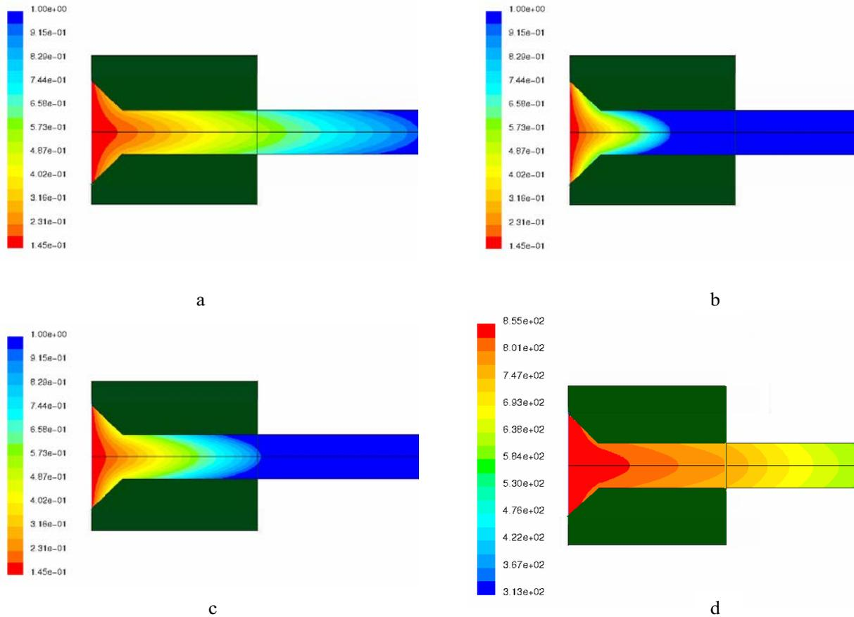
Figure 12: Comparison of solid fraction contours for different cooling conditions. The solidified shell was formed for a weak cooling condition (a), strong cooling condition (b), ideal cooling condition (c) and corresponding temperature contours (d).
