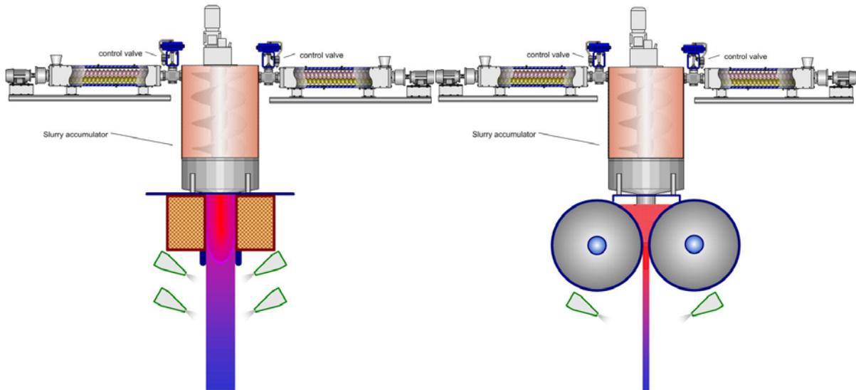
Figure 17: Conceptual designs of industrial applications of DC-rheoextrusion (left) and twin-roll rheoextrusion (right) (Scamans and Fan, 2005b, 2006b)
