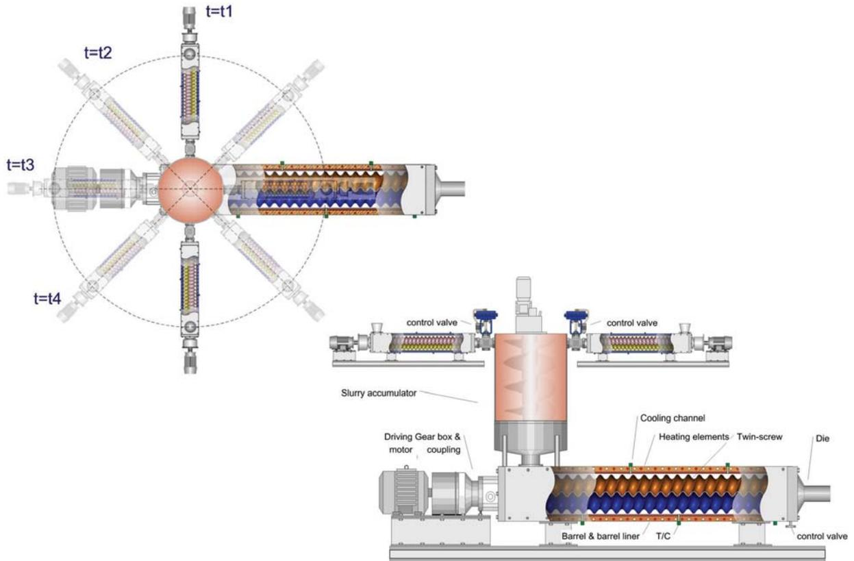
Figure 16: Schematic illustration of arrangement for rheoextrusion device (Scamans and Fan, 2006a)
