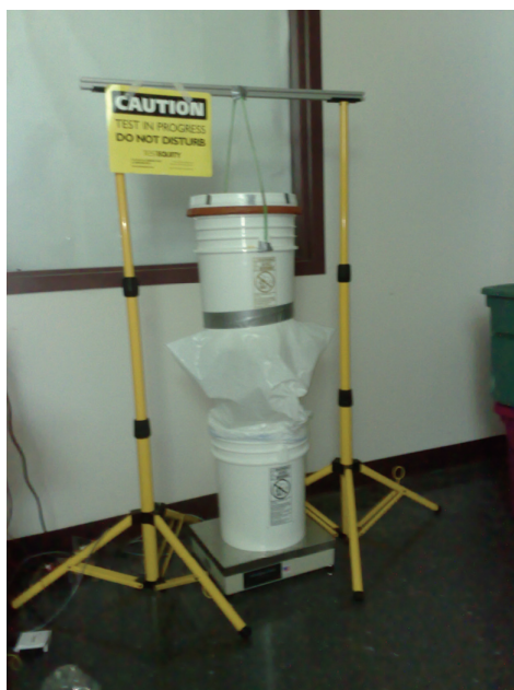
Figure 1: Model experimental setup for flow experiments conducted for different filter variants.
