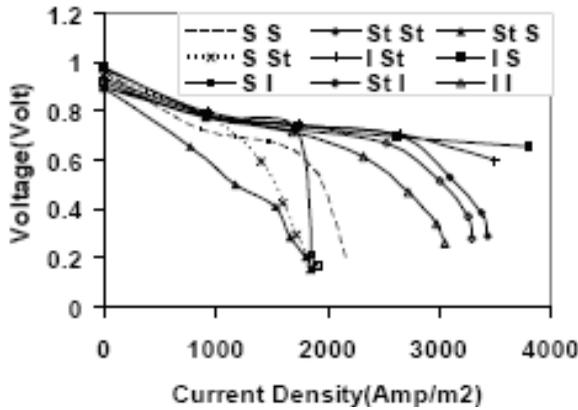
Figure 5: V-I curve at 20 sccm Hz flow rate for different gas flow channel configurations.
