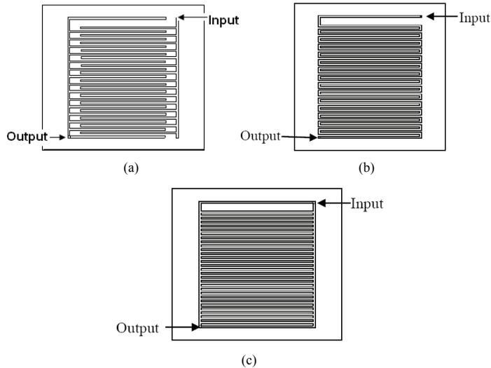
Figure 2: Gas Flow channels: (a) interdigitated (b) serpentine (c) straight design.
