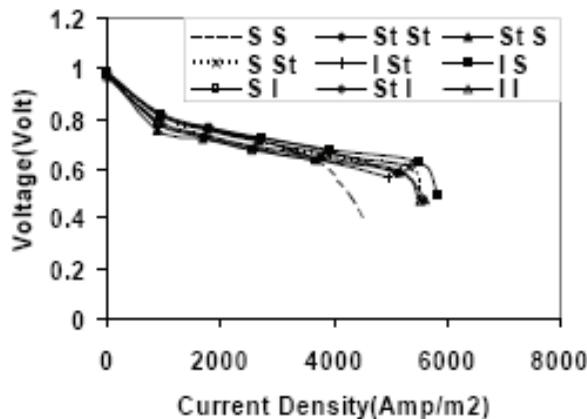
Figure 4: V-I curve at 60 sccm Hz flow rate for different gas flow channel configurations.
