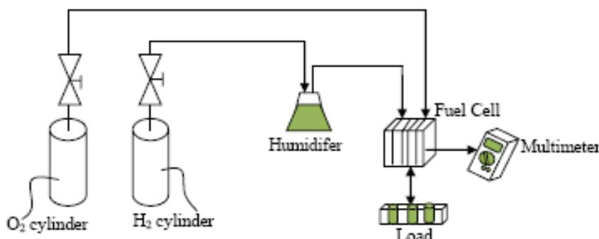
Figure 3: Experimental test stand.
