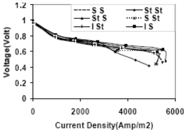
Figure 6: V-I curve at 80 sccm Hz flow rate for different gas flow channel configurations.
