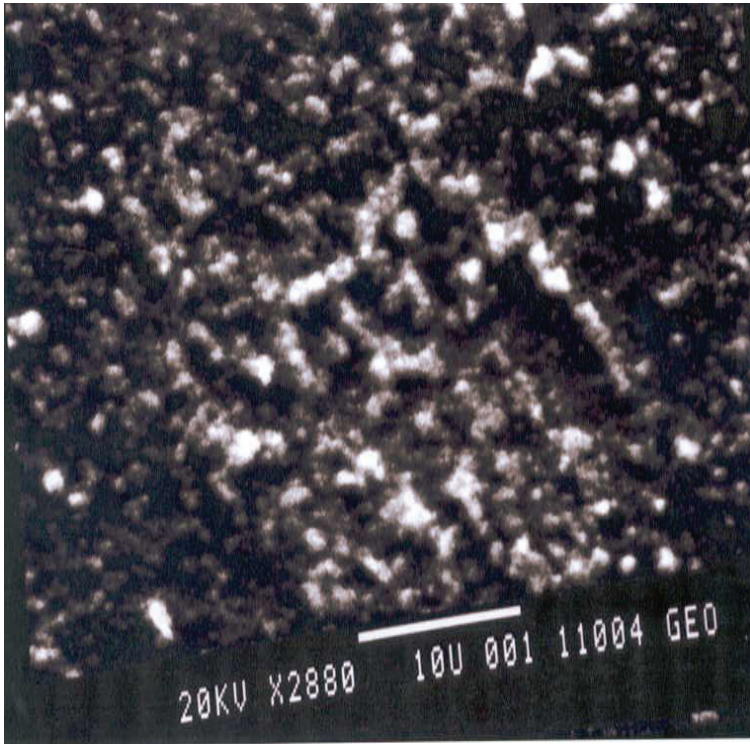
Figure 6: SEM image for one of the as-deposited ZnO thin films prepared at T_s=450^\circ\text{C} .
