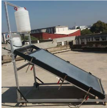
Figure 7: Cascade solar still with slope absorber plate with baffles (Fabricated at the Higher Normal School of Technical Education in Rabat)
