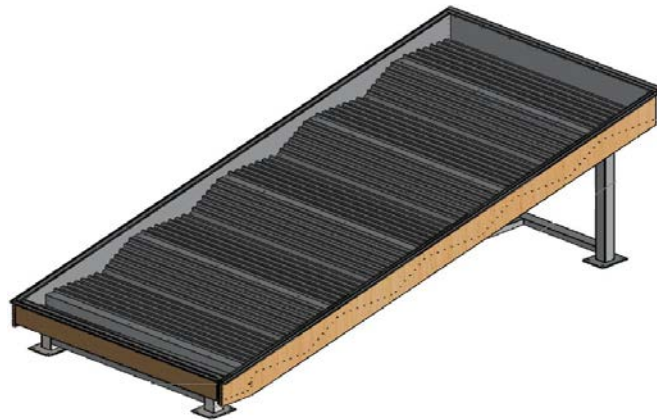
Figure 3: Cascade solar still with inclined absorber plate and baffles
