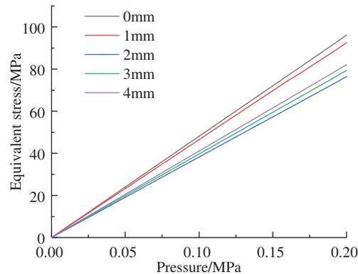
**Figure 13:** Variation of equivalent stress with different intermediate distance
