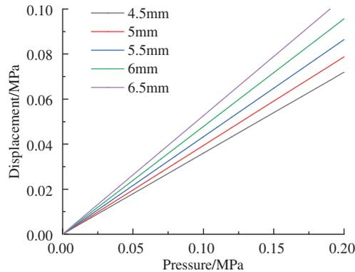
**Figure 16:** Displacement variation of wave height of different large diameter bellows
