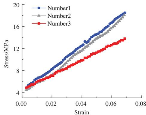
**Figure 6:** Stress-strain curve of the reducer bellows
