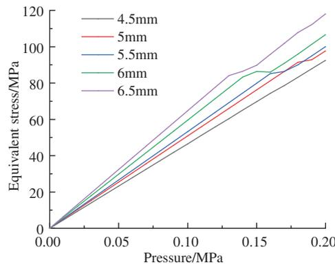
**Figure 17:** Equivalent stress variation of wave height of different large diameter bellows
