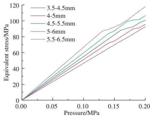
**Figure 15:** Variation of equivalent stress with different wave heights
