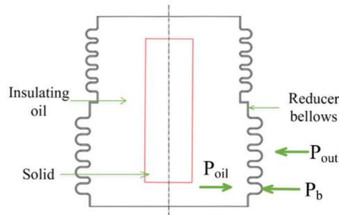
**Figure 1:** Schematic diagram of the reducer bellows
