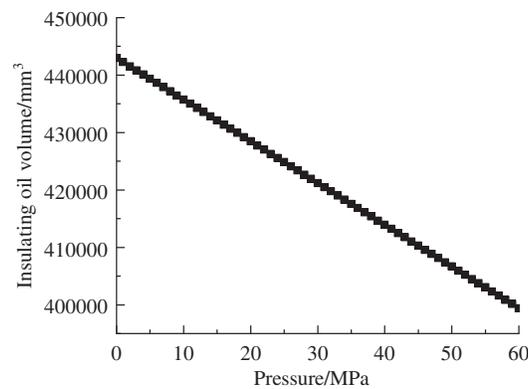
**Figure 21:** The volume of insulating oil varies with pressure
