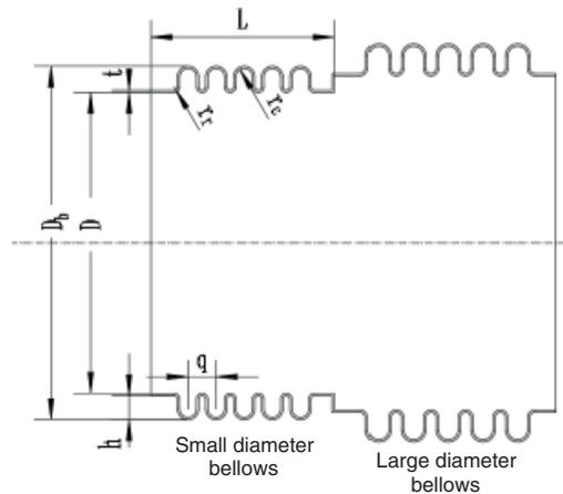
**Figure 3:** Schematic diagram of the geometric structure of the reducer bellows
