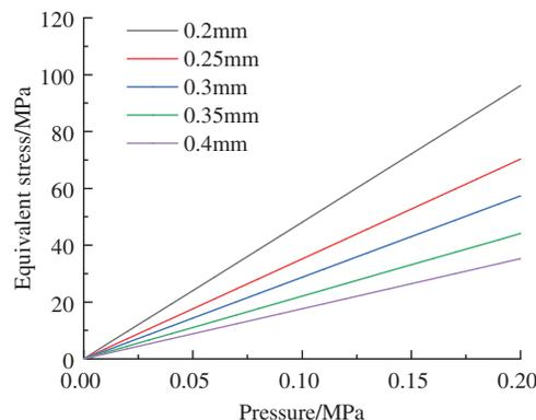
**Figure 9:** Variation of equivalent stress with different wall thicknesses
