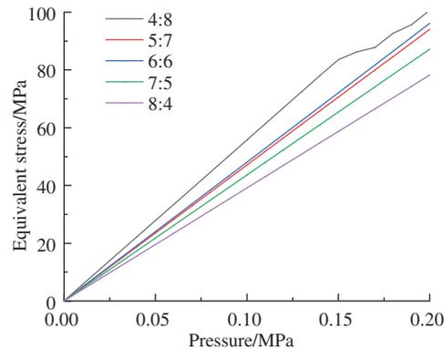
**Figure 11:** Variation of equivalent stress with different wavenumber ratios
