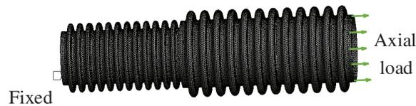
**Figure 4:** Reducer bellows finite element model
