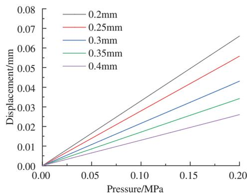
**Figure 8:** Variation of displacement with different wall thickness
