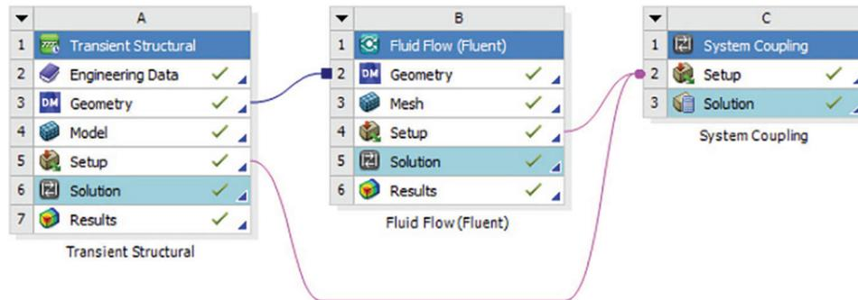
**Figure 20:** Two-way fluid-structure interaction operation settings
