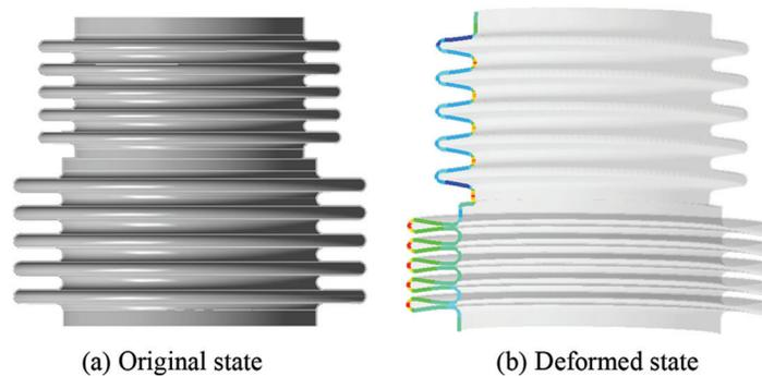
**Figure 2:** Structure diagram of the reducer bellows before and after deformation
