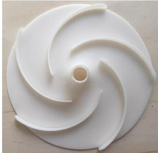
**Figure 5:** Optimized pump impeller
