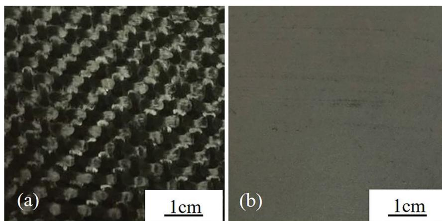
**Figure 3:** Macrograph of uncoated (a) and graphite-coated (b) 2D C/C
