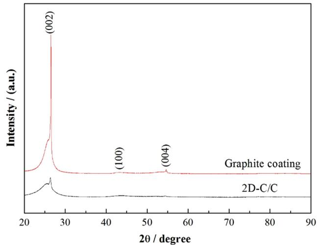
**Figure 4:** XRD results of sample and graphite coating
