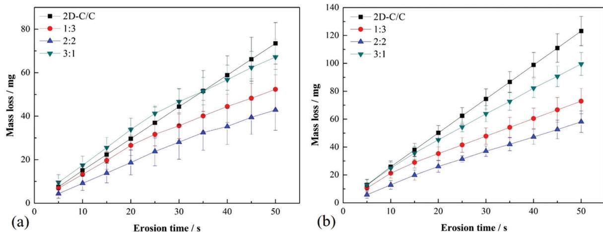
**Figure 7:** The erosion mass loss curves of graphite coating at different impact angles (a) 30° and (b) 90°
