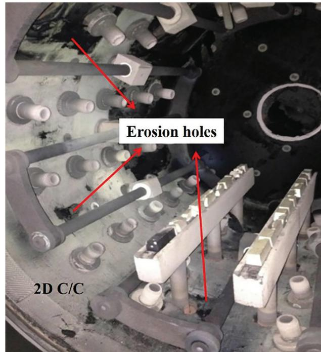
**Figure 1:** Erosion of 2D C/C composites in high-pressure gas quenching furnace
