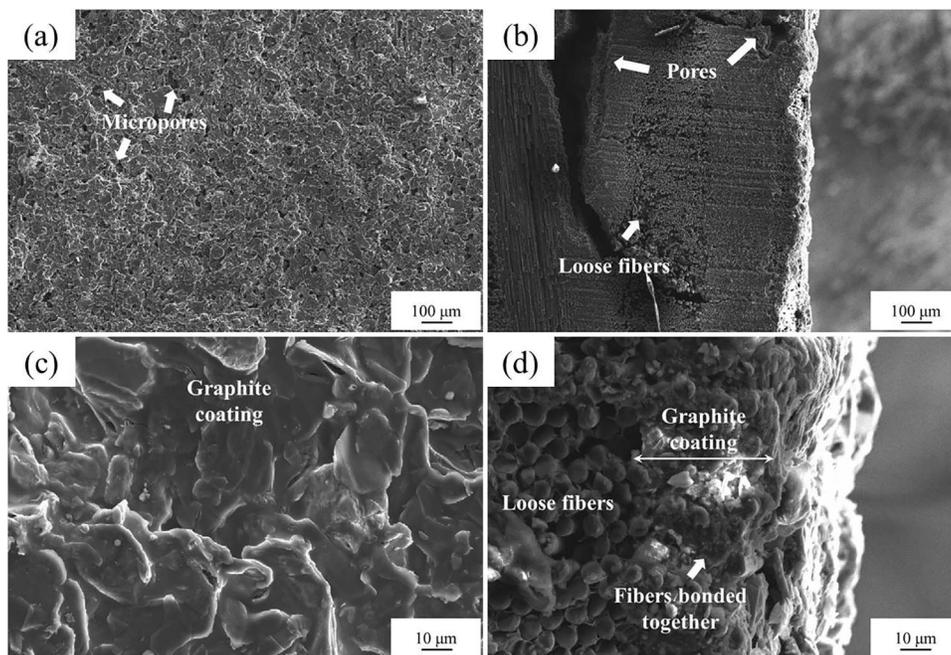
**Figure 5:** Micrographs of graphite coating: (a) and (c) surface, (b) and (d) cross-section
