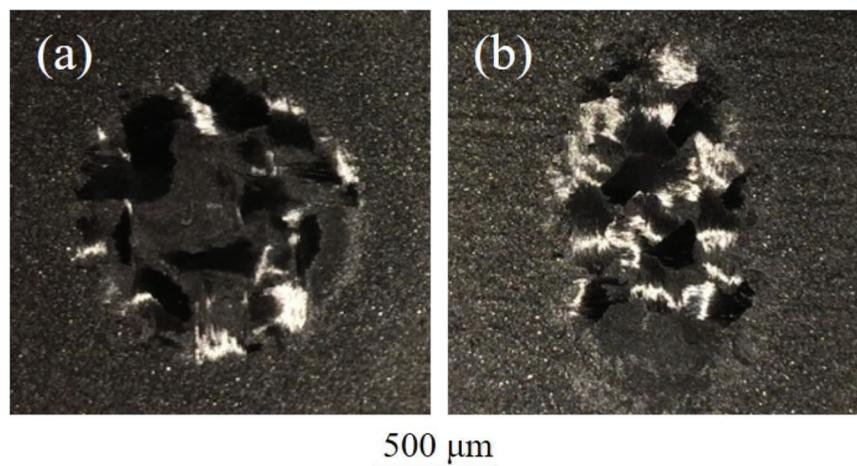
**Figure 9:** Macrographs of graphite coating for specimens after erosion at various impact angles (a)  $90^\circ$ : circle, (b)  $30^\circ$ : ellipse
