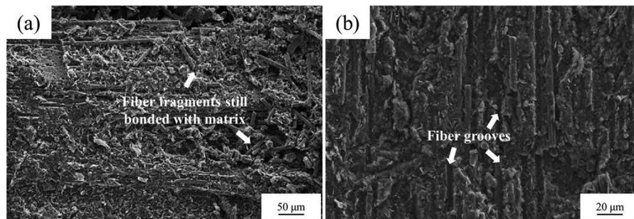
**Figure 12:** Typical micromorphology of fibers after erosion: (a) fibers fragments, and (b) fibers removal
