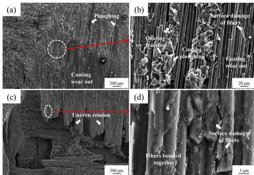
**Figure 10:** Eroded surface morphologies of specimens with graphite coating at 30° impact angle: (a) and (b) the edge of erosion scar, (c) and (d) the center of erosion scar
