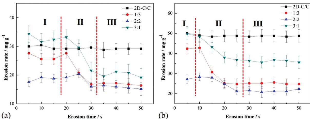
**Figure 8:** The erosion rate curves of graphite coating for C/C materials with various impact angles (a)  $30^\circ$  and (b)  $90^\circ$
