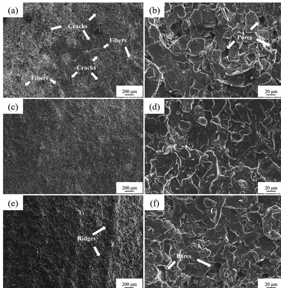
**Figure 6:** SEM images of the graphite coatings synthesized with different weight ratios of graphite powder and phenolic resin (a) and (b) 1:3, (c) and (d) 2:2, (e) and (f) 3:1
