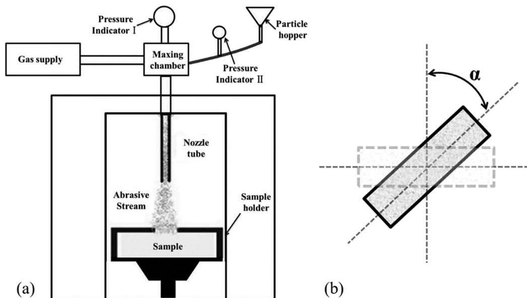
**Figure 2:** Schematic diagram of erosion device (a) and erosion angle (b)
