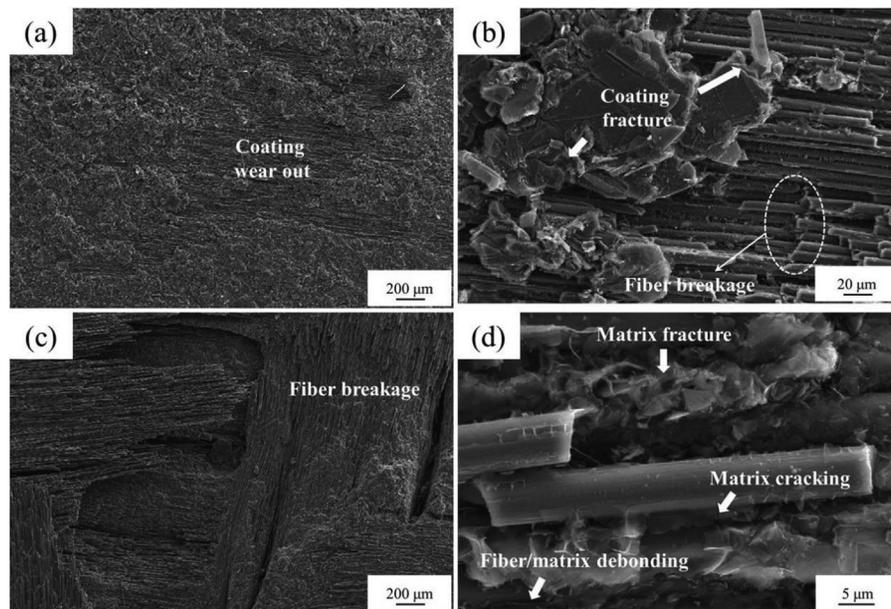
**Figure 11:** Erodent surface morphology of graphite-coated specimens at 90° impact angle: (a) and (b) the edge of erosion scar, (c) and (d) the center of erosion scar
