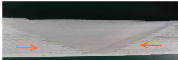
(b) Blade worn at the trailing edge
