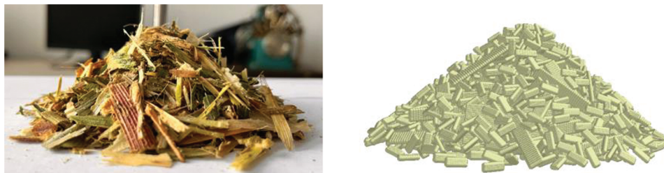
Figure 6: Comparison between crushed material and simulated heap angle tests
