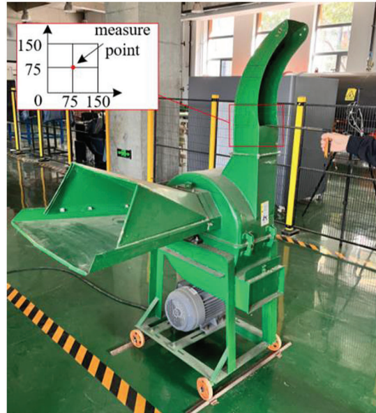
Figure 4: Airflow velocity testing
