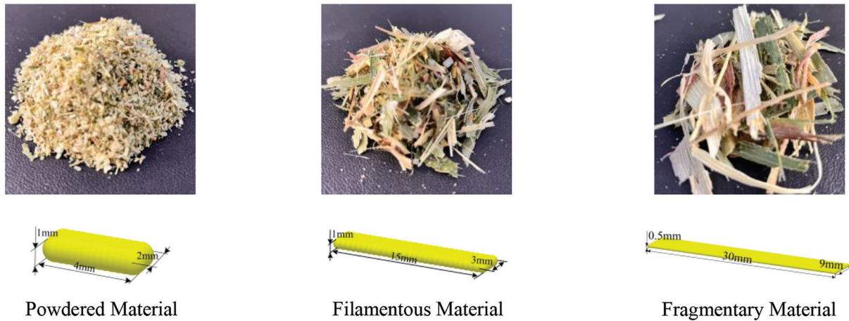
Figure 5: Comparison of crushed material and DEM model
