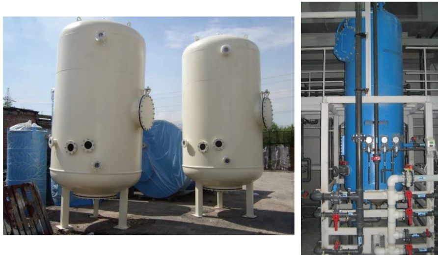
Figure 1: Industrial filter for mechanical cleaning called vertical filtration column
