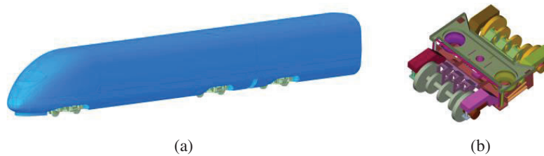
Figure 3: Geometric model: (a) train, (b) bogie
