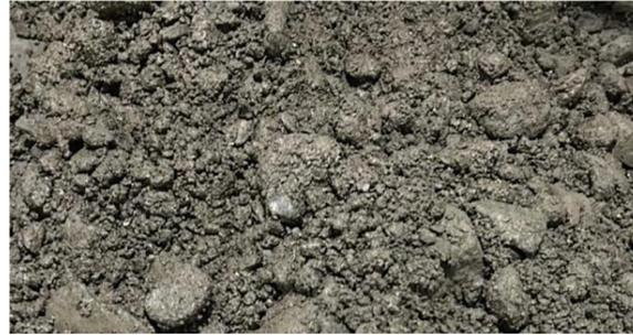
**Figure 3:** Cemented sand gravel material
