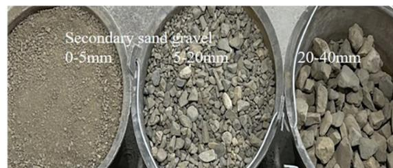
**Figure 2:** Secondary sand gravel
