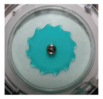
**Figure 1:** The interface between the high-viscosity glycerol colored with blue dye and the low-viscosity and denser fluid FC-40 at  $f_{rot}$  = 4.0 rps,  $f_{lib}$  = 7 Hz, and  $\varepsilon$  = 0.26. Photo is analogues to one, published in [16]
