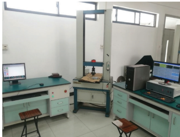
Figure 6: Image of three-point bending test equipment
