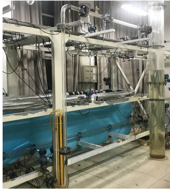
Figure 2: The GLTPF splitting experimental facility in the laboratory
