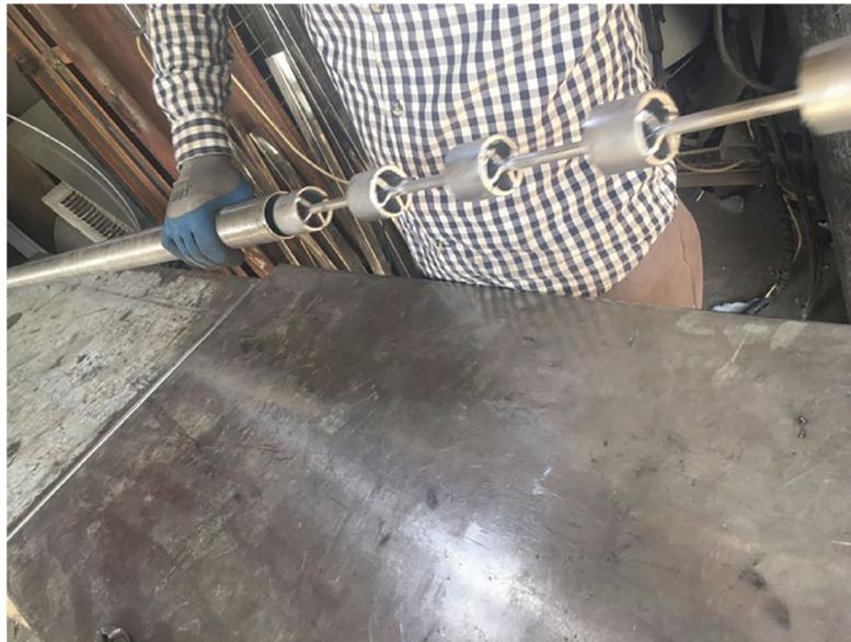
**Figure 10:** Cylindrical turbulators inside the absorber tube
