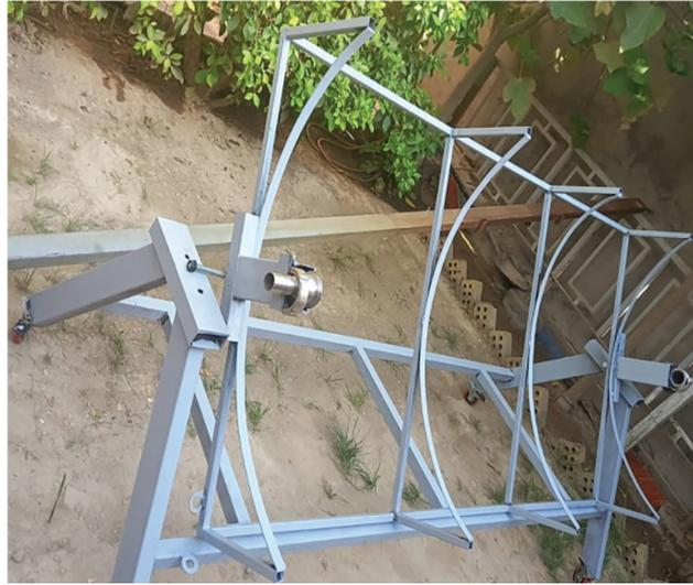
**Figure 8:** The supported structure of PTC
