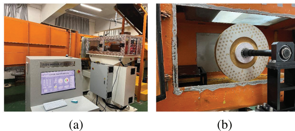
Figure 1: The setup of wind tunnel test: (a) the external view of wind tunnel and aerodynamic torque platform; (b) brake disc in wind tunnel
