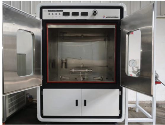
Figure 3: Core flooding apparatus
