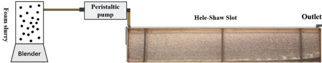
Figure 2: Dynamic sand-carrying device
