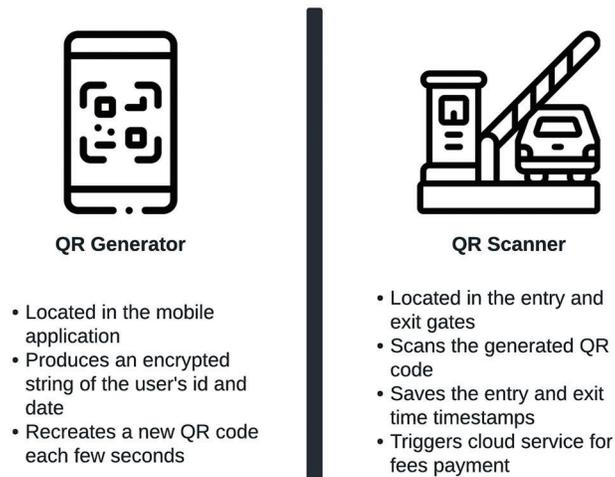
**Figure 2:** QR Generator vs. QR scanner comparison
