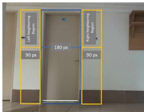
Figure 4: Constructing of neighboring regions according to a detected object's width
